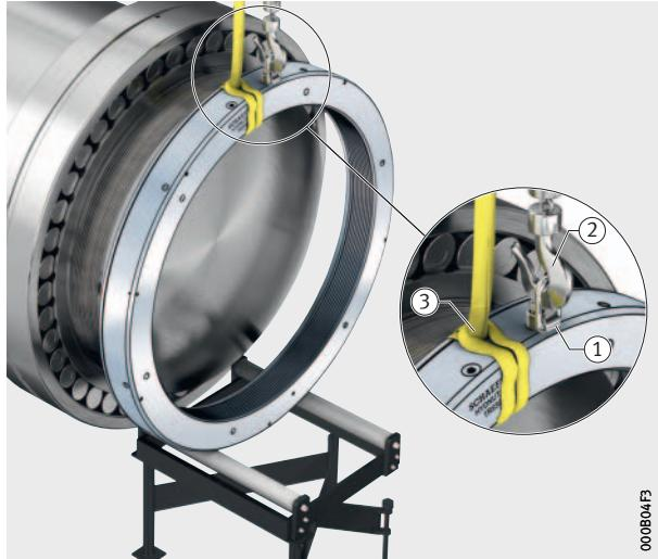
► Transport the hydraulic nut without shocks or vibration,
