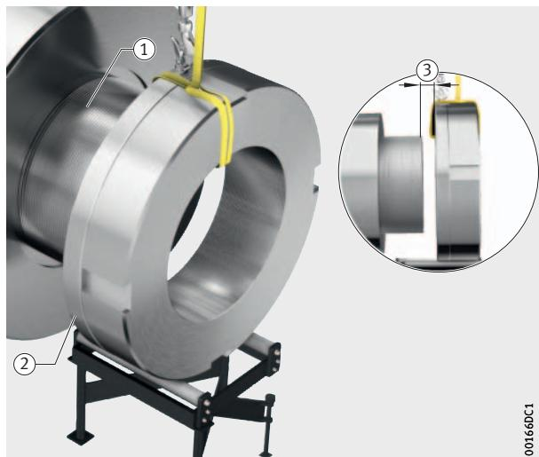
► Remove the securing belt.
