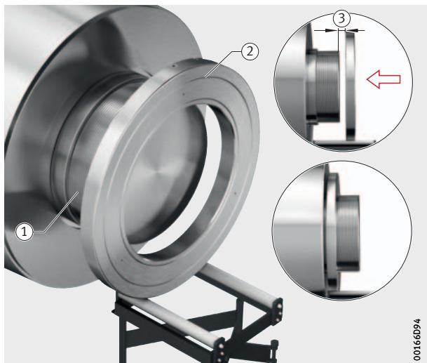
One threaded hole  $G^{1/4}$  must be located at the top, with no gap permissible between the hydraulic nut and the fixing nut or washer:
