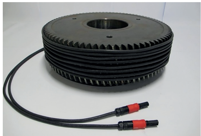
The flexible inductor is wrapped around or inside a workpiece.
