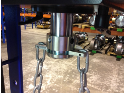
Fig. 26 Lifting chain bridge around piston head
