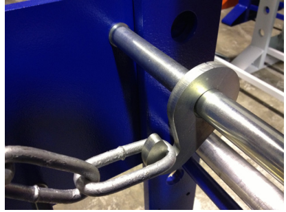
Fig. 27 Lifting chain on table hook
