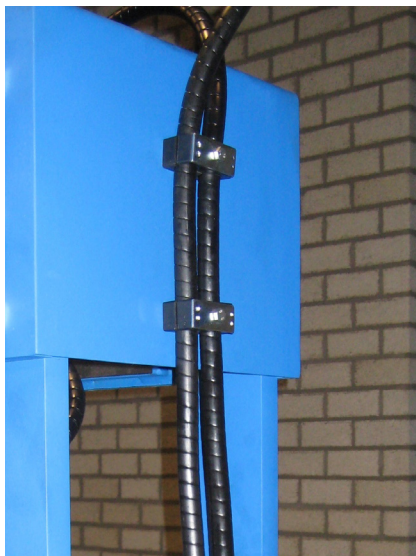
Fig. 11 Fixing hose clamps
